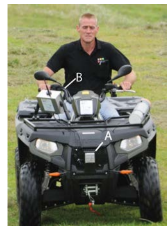
Figure 1: Feed Reader with ultrasonic head (A) and terminal (B).
